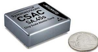
Figure 1 Chip Scale Atomic Clock developed by DARPA and commercially available through manufactures such as Symmetricom (35 grams total weight), offer affordable timing and sync capability on military vehicle platforms. 5
